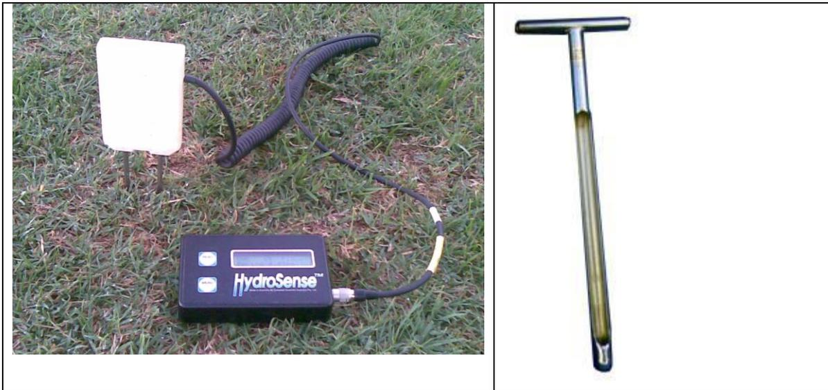
**Example of soil moisture probe (left) and soil sampler (right).**
